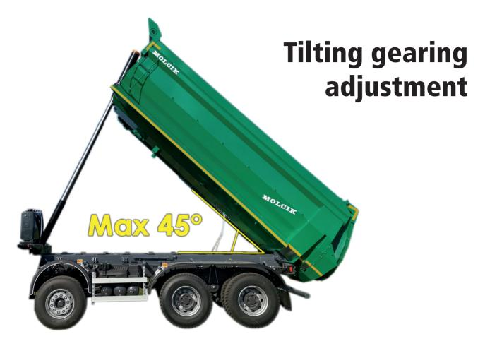
Tilting gearing is standardly set to a maximum of 45 degrees Unauthorized manipulation with the tilting gearing adjustment elements is prohibited
